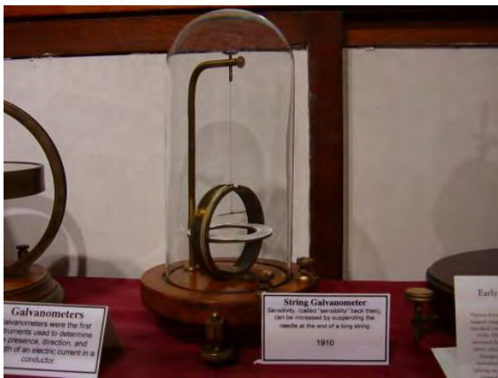
Fig. 1 (a) An antique string galvanometer, and (b) a permanent-magnet, moving coil, or PMMC movement.
