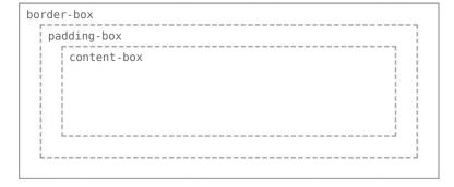
Figure 4.6 Different boxsizing values allow the width of an element—and its box—to be calculated from different areas
