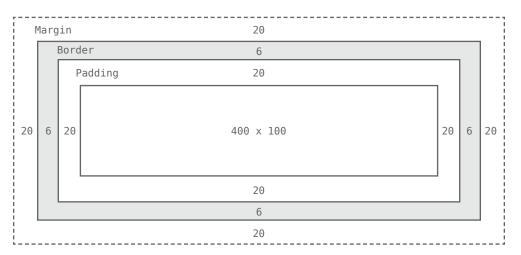
Figure 4.3 The box model broken down, including a base height and width plus paddings, borders, and margins
