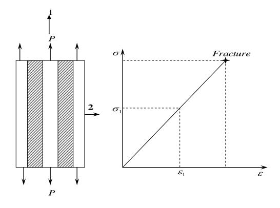
Fig.1.4 Unidirectional lamina loaded in the fiber-direction
