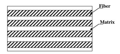
Fig. 1.1 Structure of a fibrous composite
