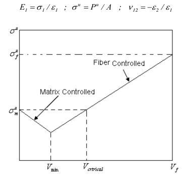
Fig. 1.3 Variation of unidirectional lamina strength with the fiber volume fraction
