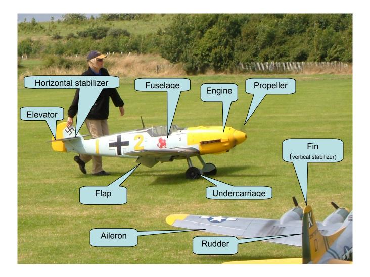
**AILERON** - Hinged control surface located on the back of the wing, furthest from the fuselage. When the servo moves the aileron via the pushrods, the plane is capable of turning and rolling.
