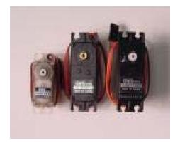
A servo is a small motor wired to the receiver in the airplane. The receiver decodes the signals from the transmitter and instructs the servo to move a certain amount. This movement is transmitted to the aircraft's control surfaces--usually by the pushrods connecting them to the servo.
