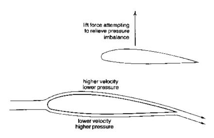
Newton's laws state that for every action there is an equal and opposite reaction and the alternative explanation is as follows.
