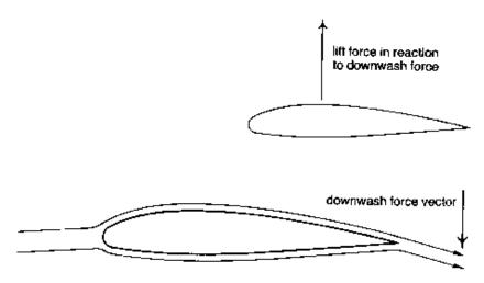
The airfoil shape of the wing causes the flow of air to be deflected downwards – and this is the importance of the airfoil shape of the wing which causes this deflection which is necessary for either of our two scientist's theories to hold good. Therefore there must be a reaction in the opposite direction which is equal in force to the force of the downwash – and this is lift.
