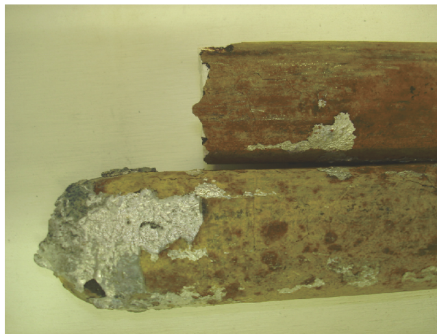
Figure 1: Discoloration and accumulation of material on a bone ash coated flow control pin.
