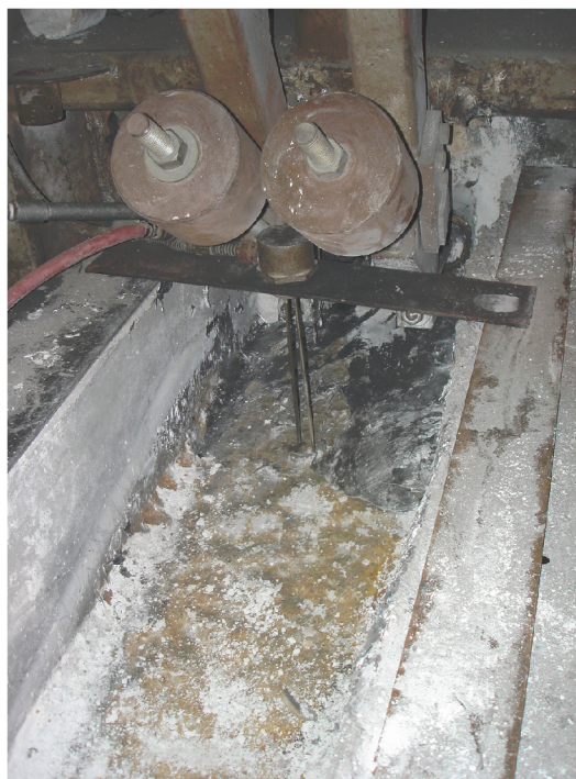
Figure 4: Discoloration of base of transfer launder due to metal phosphide formation.
