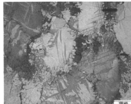
Figure 11: Representative microstructure of the thixocast MEZ alloy after creep at 175°C and 100 MPa, optical microscopy.
