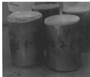
Figure 3 – Precursor material produced by cold compaction of rapid solidified powders made of BAS materials.
