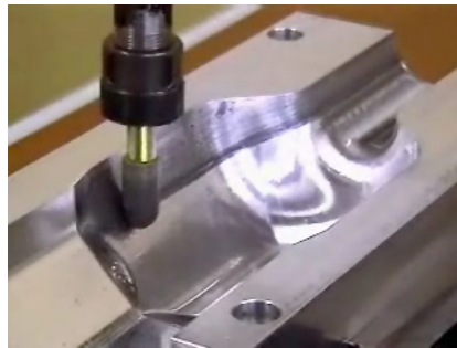
Figure 1.19. Polishing scene of PET bottle mold
