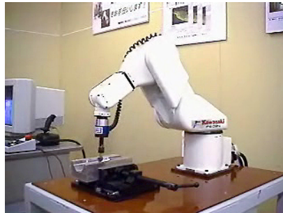
Figure 1.18. Mold-polishing robot developed based on KAWASAKI FS03
