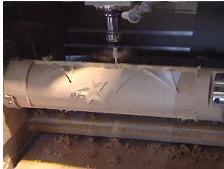
Figure 1.7. Machining scene of a wooden paint roller
