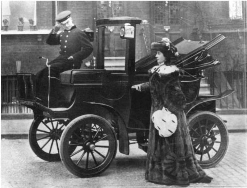
Figure 1.5 New York taxi cab in about 1901, a battery electric vehicle (The lady in the picture is Lily Langtree, actress and mistress of King Edward VIII)
