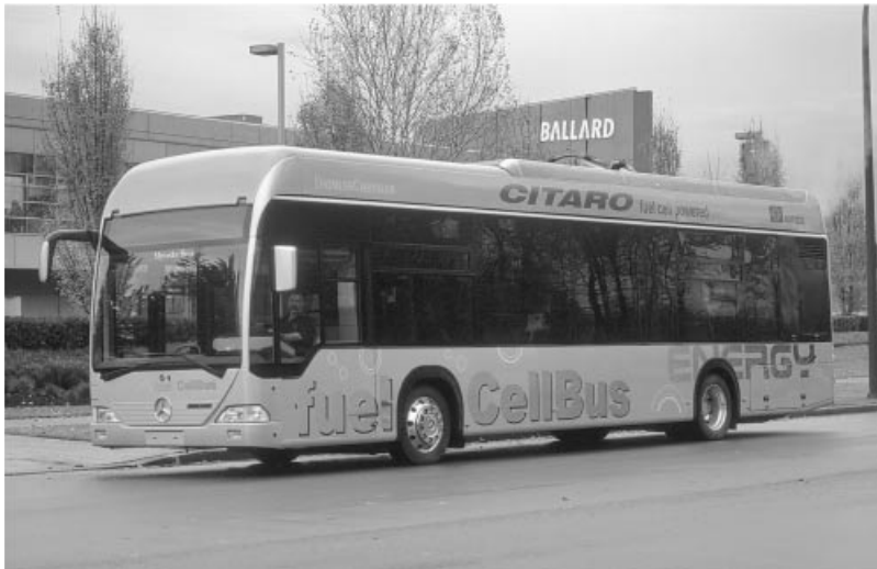
Figure 1.17 Citro fuel-cell-powered bus, one of a fleet that entered service in 2003 (Photograph reproduced by kind permission of Ballard Power Systems)
