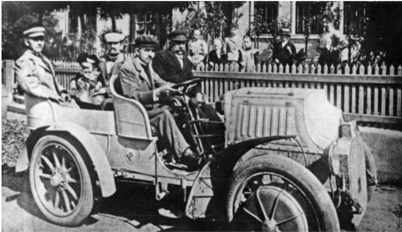
Figure 1.7 The Lohner Porshe, the first electric hybrid vehicle designed and driven by Dr Ferdinand Porsche (Reproduced with permission from the Beaulieu Motor Museum)
