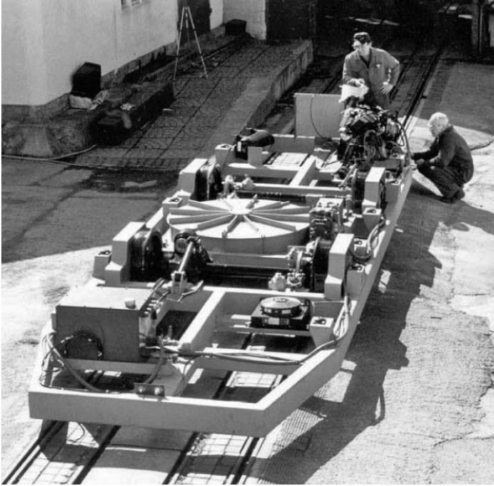
Figure 2.7 ‘Parry People Mover’ chassis. The enclosed flywheel can be clearly seen in the middle of the vehicle (Photograph kindly supplied by Parry People Movers Ltd)
