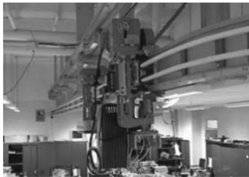
Figure 4.5 Inductively powered monorail system (Reproduced by kind permission of Department of Electrical and Computer Engineering the University of Auckland)
