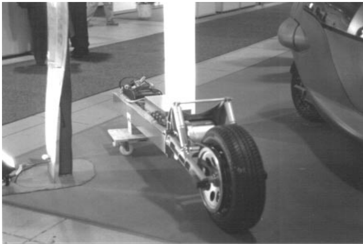
Figure 9.11 This power module comprises motor, controller, battery and one driven wheel in a neat unit that could be built into a wide range of vehicle designs
