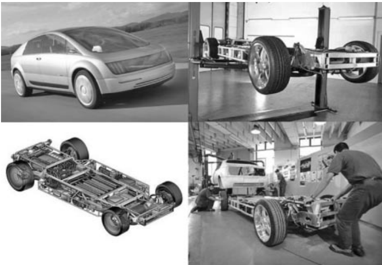
Figure 9.16 GM's 'Hy-wire' chassis and one-body design (Reproduced by kind permission of General Motors Corp.)
