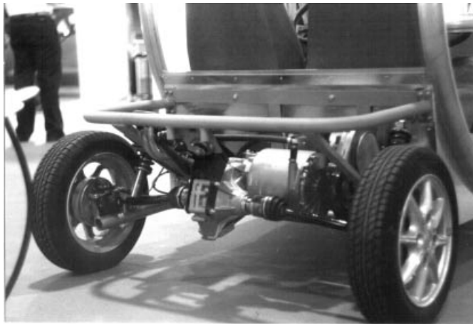
Figure 9.7 Example of type (a) of Figure 9.6 on an experimental electric vehicle by MES-DES SA. The mounting of the motor is transverse, so there is no drive shaft
