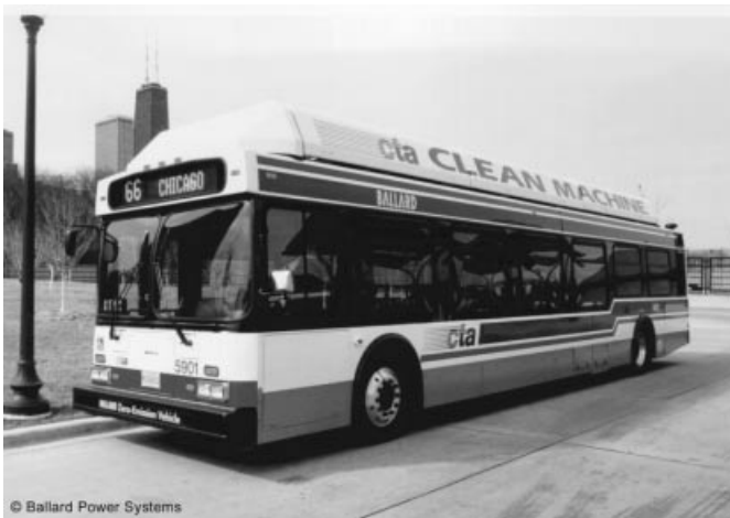
Figure 14.6 Fuel-cell-powered bus, 1998 model. (Reproduced by kind permission of Ballard Power Systems.)
