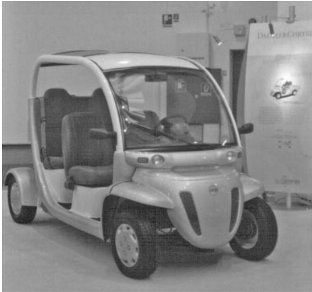
Figure 14.3 An example of the ‘low-speed vehicle’ (LSV) type of electric car
