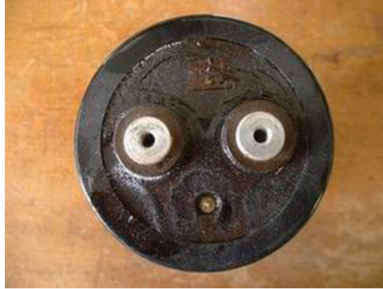
Figure 18.20. View from above of a capacitor presenting electrolyte leakage
