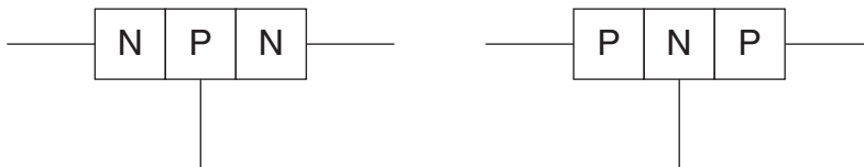
FIGURE 3.5 Smash diodes together to make a transistor.
