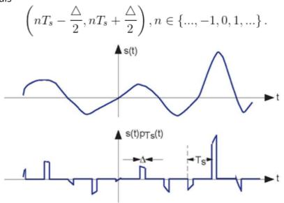
**Figure 5.3 Sampled Signal** The waveform of an example signal is shown in the top plot and its sampled version in the bottom.
