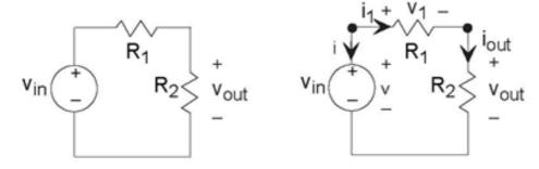
Figure 3.7 Simple circuit The circuit shown is perhaps the simplest circuit that performs a signal processing function. The input is provided by the voltage source  $v_{in}$  and the output is the voltage  $v_{out}$  across the resistor labelled  $R_2$ .
