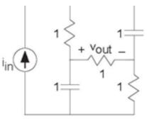
Figure 3.77 A Simple Circuit
