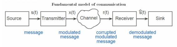
Figure 1.4 The Fundamental Model of Communication.
