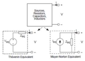
(b) Equivalent circuits with impedances.
