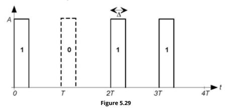
This signal (Figure 5.29) serves as the input to a first-order RC lowpass filter. We want to design the filter and the parameters  $\Delta$  and T so that the output voltage at time 4T (for a 4-bit converter) is proportional to the number. This combination of pulse creation and filtering constitutes our simple D/A converter. The requirements are
