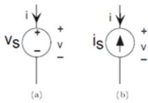
**Figure 3.5 Sources** The voltage source on the left and current source on the right are like all circuit elements in that they have a particular relationship between the voltage and current defined for them. For the voltage source, v = vs for any current i; for the current source, i = -is for any voltage v
