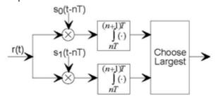
Figure 6.14 Optimal receiver structure
