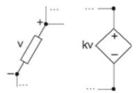
**Figure 3.39 dependent sources** Of the four possible dependent sources, depicted is a voltage-dependent voltage source in the context of a generic circuit.
