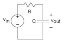
Figure 3.29 A simple RC circuit
