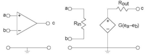
**Figure 3.40 op-amp** The op-amp has four terminals to which connections can be made. Inputs attach to nodes a and b, and the output is node c. As the circuit model on the right shows, the op-amp serves as an amplifier for the difference of the input node voltages.
