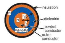
Figure 6.1 Coaxial Cable Cross-section
