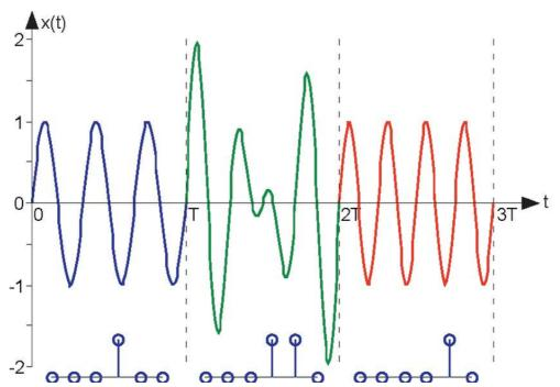
**Figure 4.9 Encoding Signals** The encoding of signals via the Fourier spectrum is shown over three "periods." In this example, only the third and fourth harmonics are used, as shown by the spectral magnitudes corresponding to each **7**-second interval plotted below the waveforms. Can you determine the phase of the harmonics from the waveform?
