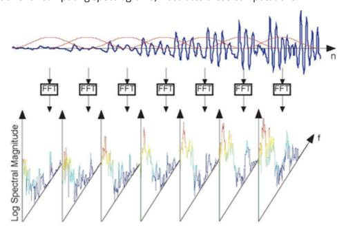
Figure 5.17 Overlapping windows for computing spectrograms
