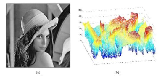
**Figure 1.2 Lena** On the left is the classic Lena image, which is used ubiquitously as a test image. It contains straight and curved lines, complicated texture, and a face. On the right is a perspective display of the Lena image as a signal: a function of two spatial variables. The colors merely help show what signal values are about the same size. In this image, signal values range between 0 and 255; why is that?
