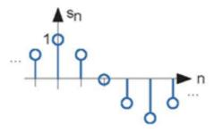
**Figure 2.7 Discrete-Time Cosine Signal** The discrete-time cosine signal is plotted as a stem plot. Can you find the formula for this signal?
