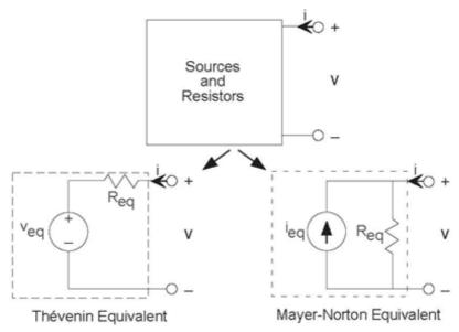
**Figure 3.20 Thevenin and Mayer-Norton equivalent** All circuits containing sources and resistors can be described by simpler equivalent circuits. Choosing the one to use depends on the application, not on what is actually inside the circuit.
