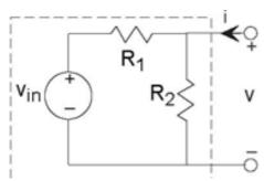
Figure 3.16 Simple attenuator circuit
