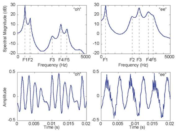
**Figure 4.15 Speech Spectrum** The ideal frequency response of the vocal tract as it produces the sounds "oh" and "ee" are shown on the top left and top right, respectively. The spectral peaks are known as formants, and are numbered consecutively from low to high frequency. The bottom plots show speech waveforms corresponding to these sounds.
