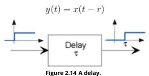
Here,  $\tau$  is the delay. The way to understand this system is to focus on the time origin: The output at time  $t = \tau$  equals the input at time t = 0. Thus, if the delay is positive, the output emerges later than the input, and plotting the output amounts to shifting the input plot to the right. The delay can be negative, in which case we say the system **advances** its input. Such systems are difficult to build (they would have to produce
