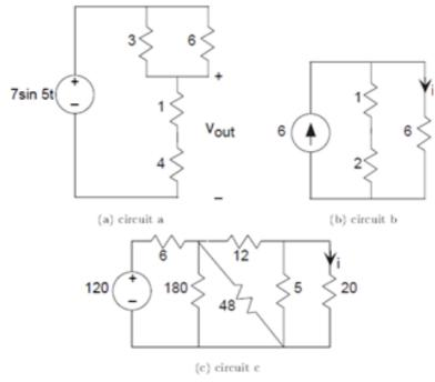
Figure 3.56 Current and Voltage Divider
