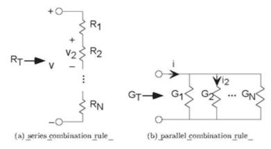
Figure 3.15 Series and parallel combonation rules
