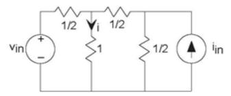
Figure 3.55 Superposition Principle
