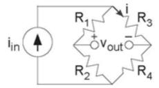
Figure 3.59 Bridge Circuits
