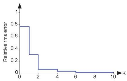
**Figure 4.6 Approximation error for a half-wave rectified sinusoid**: The rms error calculated according to (4.25) is shown as a function of the number of terms in the series for the half-wave rectified sinusoid. The error has been normalized by the rms value of the signal.
