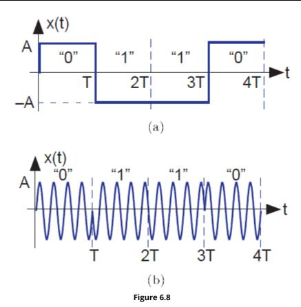
The upper plot shows how a baseband signal set for transmitting the bit sequence 0110. The lower one shows an amplitude-modulated variant suitable for wireless channels.
