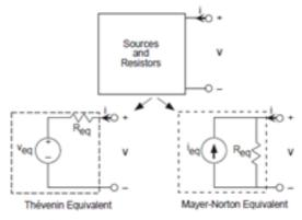
(a) Equivalent circuits with resistors.
