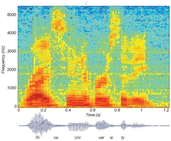
**Figure 4.17 spectrogram** Displayed is the spectrogram of the author saying "Rice University." Blue indicates low energy portion of the spectrum, with red indicating the most energetic portions. Below the spectrogram is the time-domain speech signal, where the periodicities can be seen.
