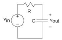
Figure 3.23 A simple RC circuit
