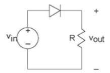
Figure 3.49 diode circuit
