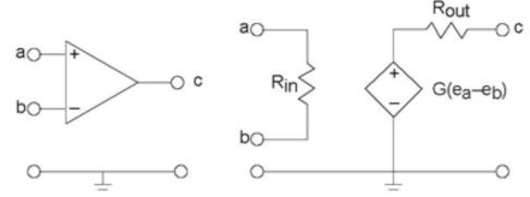
**Figure 3.42 Op-Amp** The op-amp has four terminals to which connections can be made. Inputs attach to nodes a and b, and the output is node c. As the circuit model on the right shows, the op-amp serves as an amplifier for the difference of the input node voltages.
