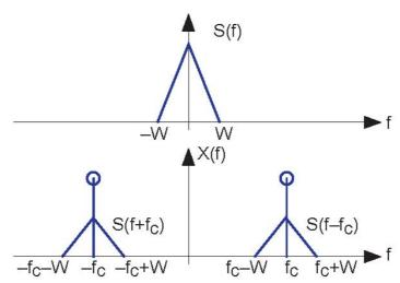
**Figure 4.12 Spectrum of the amplitude modulated signal** A signal which has a triangular shaped spectrum is shown in the top plot. Its highest frequency the largest frequency containing power is **W** Hz. Once amplitude modulated, the resulting spectrum has "lines" corresponding to the Fourier series components at  $\pm (f_c)$  and the original triangular spectrum shifted to components at  $\pm (f_c)$  and scaled by .
