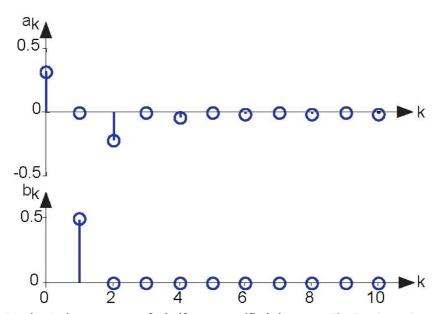
**Figure 4.3 Fourier Series spectrum of a half-wave rectified sine wave** The Fourier series spectrum of a half-wave rectified sinusoid is shown. The index indicates the multiple of the fundamental frequency at which the signal has energy.
