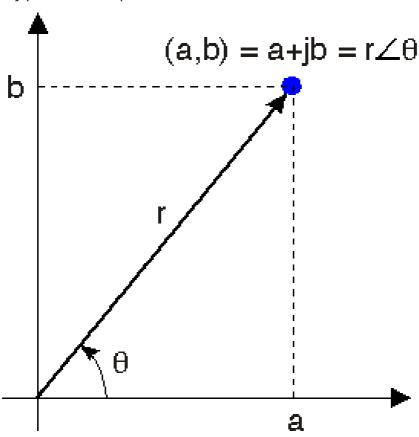
**Figure 2.1 The Complex Plane** A complex number is an ordered pair (a,b) that can be regarded as coordinates in the plane. Complex numbers can also be expressed in polar coordinates as  $r \angle \theta$ .
