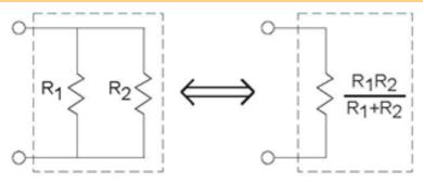
Figure 3.11 A parallel combination of resistors
