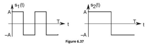
Thus, bits are represented in data stream 1 by  $s_1(t)$  and  $-s_1(t)$  and in data stream 2 by  $s_2(t)$  and  $-s_2(t)$ , each of which are modulated by 900 MHz carrier. The transmitter sends the two data streams so that their bit intervals align. Each receiver uses a matched filter for its receiver. The requirement is that each receiver **not** receive the other's bit stream.
