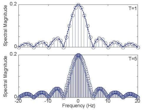
**Figure 4.11 Spectrum** The upper plot shows the magnitude of the Fourier series spectrum for the case of T =1 with the Fourier transform of p(t) shown as a dashed line. For the bottom panel, we expanded the period to T =5, keeping the pulse's duration fixed at 0.2, and computed its Fourier series coefficients.
