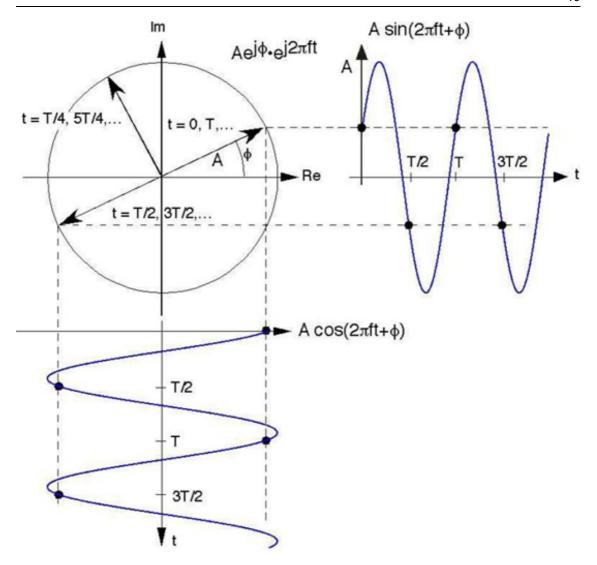
**Figure 2.2 The complex exponential** Graphically, the complex exponential scribes a circle in the complex plane as time evolves. Its real and imaginary parts are sinusoids. The rate at which the signal goes around the circle is the frequency f and the time taken to go around is the period T . A fundamental relationship is T = f 1.
