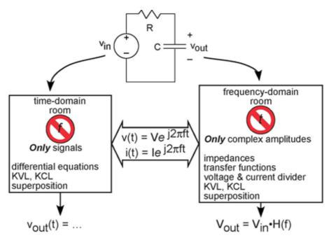
**Figure 3.25 Two Rooms** The time and frequency domains are linked by assuming signals are complex exponentials. In the time domain, signals can have any form. Passing into the frequency domain "work room," signals are represented entirely by complex amplitudes.
