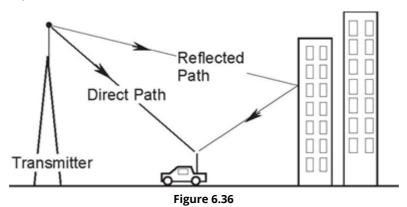
Assume that the length of the direct path is *d* meters and the reflected path is 1.5 times as long. What is the model for the channel, including the multipath and the additive noise?
