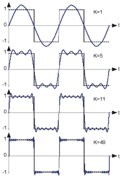
**Figure 4.8 Fourier series approximation of a square wave** Fourier series approximation to sq (t). The number of terms in the Fourier sum is indicated in each plot, and the square wave is shown as a dashed line over two periods.
