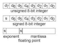
**Figure 5.2 Number representations on computers** The various ways numbers are represented in binary are illustrated. The number of bytes for the exponent and mantissa components of foating point numbers varies.
