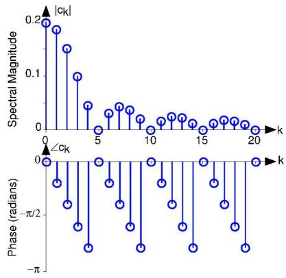
**Figure 4.2 Periodic Pulse Sequence** The magnitude and phase of the periodic pulse sequence's spectrum is shown for positive frequency indices. Here =0.2 and A =1.
