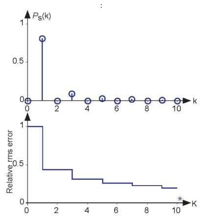
**Figure 4.7 Power spectrum and approximation error for a square wave** The upper plot shows the power spectrum of the square wave, and the lower plot the rms error of the fnite-length Fourier series approximation to the square wave. The asterisk denotes the rms error when the number of terms **K** in the Fourier series equals 99.
