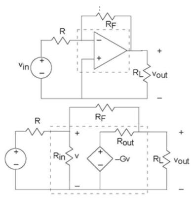
**Figure 3.41 feedback op-amp** The top circuit depicts an op-amp in a feedback amplifier configuration. On the bottom is the equivalent circuit, and integrates the op-amp circuit model into the circuit.
