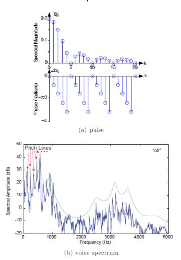
**Figure 4.16 voice spectrum** The vocal tract's transfer function, shown as the thin, smooth line, is superimposed on the spectrum of actual male speech corresponding to the sound "oh." The pitch lines corresponding to harmonics of the pitch frequency are indicated. (a) The vocal cords' output spectrum P<sub>T</sub> (f).
