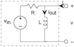
Figure 3.31 RL circuit
