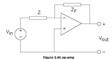
$$\frac{V_{out}}{V_{in}} = -\left(\frac{Z_F}{Z}\right)$$
