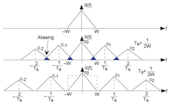
**Figure 5.4 aliasing** The spectrum of some bandlimited (to  $\mathbf{W}$  Hz) signal is shown in the top plot. If the sampling interval  $\mathbf{T}_S$  is chosen too large relative to the bandwidth  $\mathbf{W}$ , aliasing will occur. In the bottom plot, the sampling interval is chosen sufficiently small to avoid aliasing. Note that if the signal were not bandlimited, the component spectra would always overlap.
