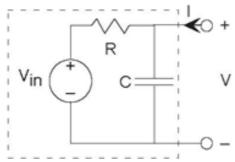
Figure 3.28 Simple RC Circuit
