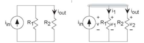
Figure 3.10 A simple parallel circuit.
