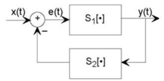
Figure 2.12 The feedback configuration.
