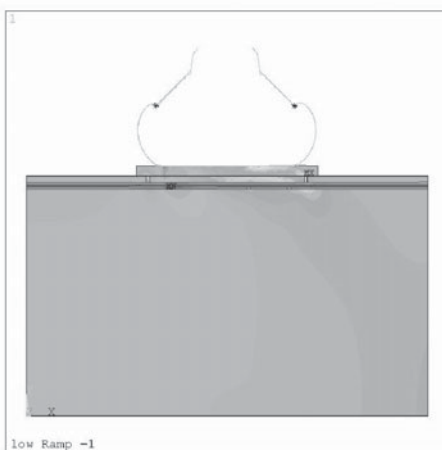
FIGURE 11-22 Maximum principal stresses in die versus bond pad thickness at the first step of cycle 6 (capillary toward left).
