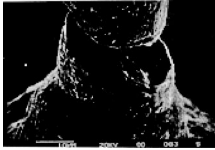
FIGURE 3B-2 A temperature cycled Cu ball bond (encapsulated) that developed a neck crack.
