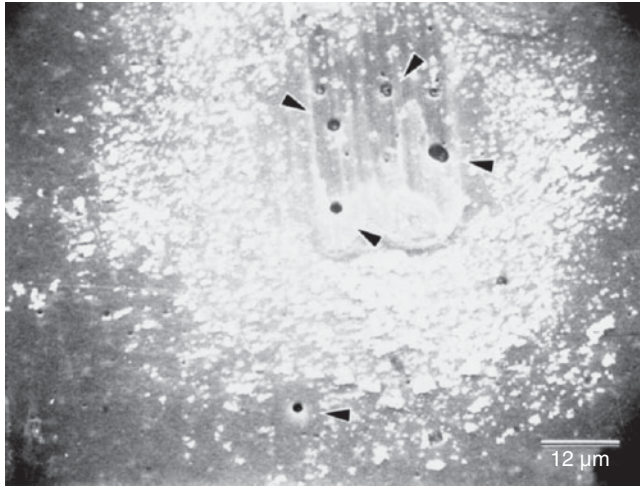
FIGURE 5-13 Scanning electron micrograph of pitted Al-1.5% Cu bonding pads following ball shearing showing the lack of bonding (i.e., no Au residue or any evidence of bonding) in the corrosion halo areas as compared with the normal areas. (After Thomas [5-68] 67; © IEEE.)
