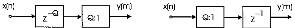
Figure 2.15 Q -units of Delay and Q -to-1 Down Sampler Is Equivalent to Q -to-1 Down Sampler and 1-unit of Delay.
