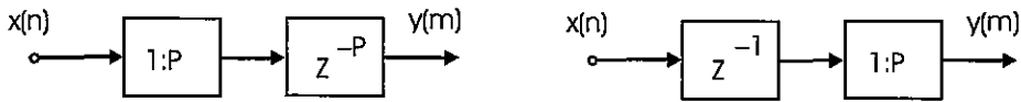
Figure 2.16 1-to-P Up Sampler Followed by P-Units of Delay Is Equivalent to 1-Unit of Delay and P-to-1 Up Sampler.
