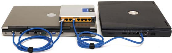
Figure 6-3 A switch connected by UTP cable to two PCs
