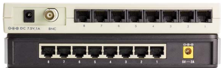
Figure 4-24 Hub (top) and switch (bottom) comparison
