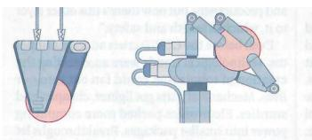
Flexible flaps Soft, lightweight, and flexible flaps use electrostatic forces to pick up a fragile object. **High-speed claw** This robot hand-fastest on the planet-can catch an object in five-hundredths of a second. Humanoid hand This robot has ultrasensitive touch sensors and moves much like a human hand does. **Biomimetic hand** It mimics the human hand with artificial joint capsules and rubber ligaments and tendons.
