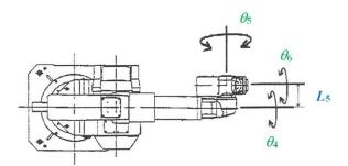
Fanuc S10 offset 3-dof roll-pitch-roll wrist
