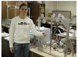
3-dof Cable-Suspended Haptic Interface
