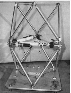
NASA Variable Geometry Truss
