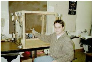
8-dof Cable-Suspended Haptic Interface
