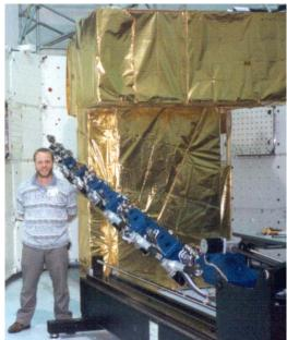
NASA KSC 18-dof Serpentine Truss Manipulator
