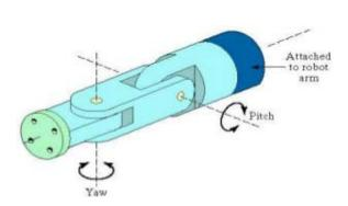
Offset 2-dof pitch-yaw wrist for axisymmetric tasks
