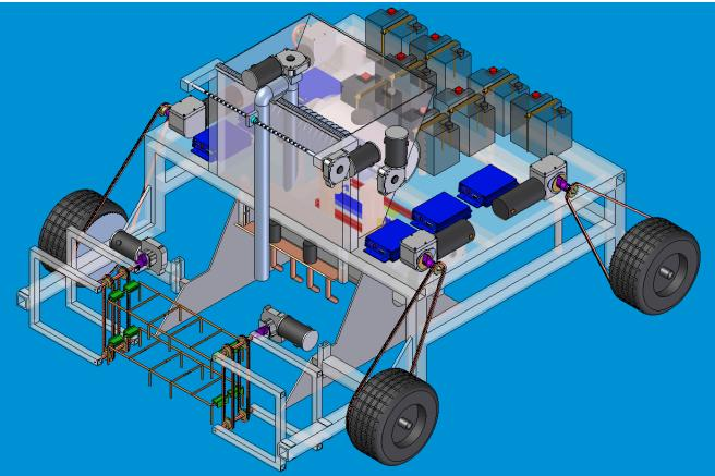
4-dof Autonomous Concrete-Paving Mobile Robot
