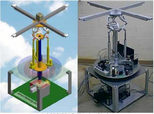
4-dof GPS/IMU Calibration Platform
