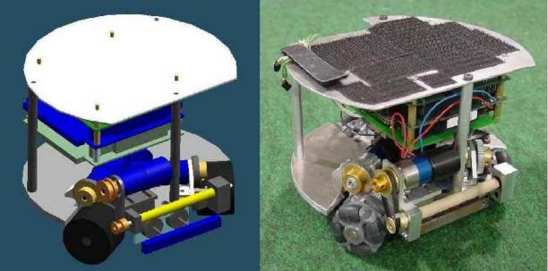
3-dof Omni-Directional RoboCup Wireless Autonomous Mobile Robot
