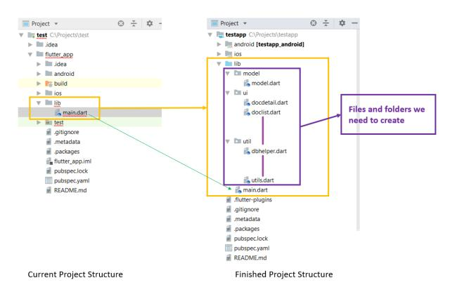
Figure 2-d: The app's project folder structure comparison
