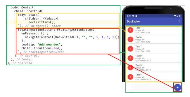
Figure 4-d: The main screen's body
