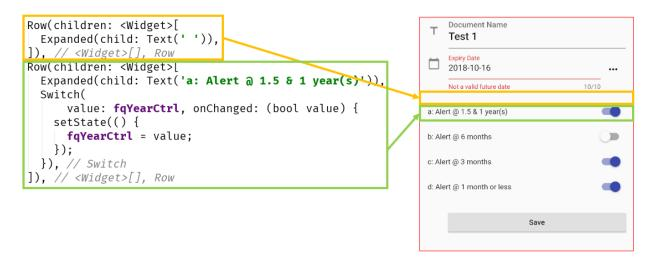
Figure 3-p: The empty row and first alert field—Document Details screen
