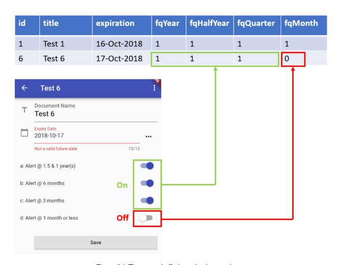
Figure 3-j: The on and off alerts database values
