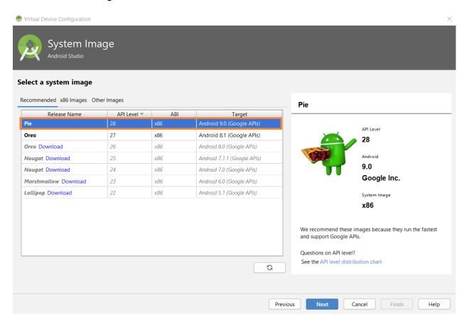
Figure 1-k: Creating a virtual device (step 3)
