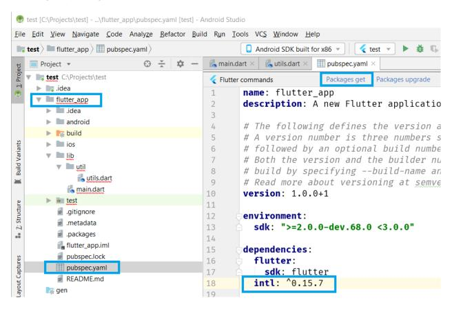
Figure 2-j: Adding the package to Pubspec.yaml
