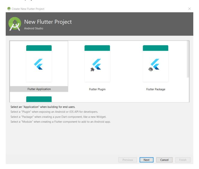
Figure 1-f: Create new Flutter project option (step 1)
