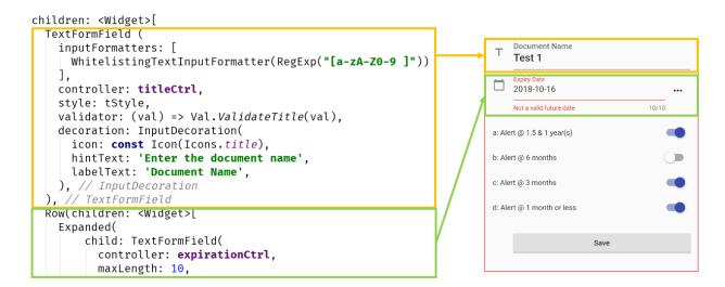
Figure 3-n: The first two data-entry widgets—Document Details screen
