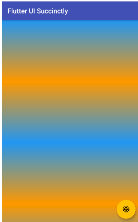
Figure 3-t: A Container Widget with a LinearGradient – Mirror TileMode
