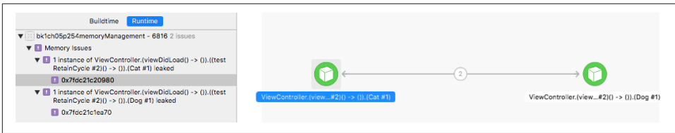
Figure 9-18. The memory graph displays a leak
