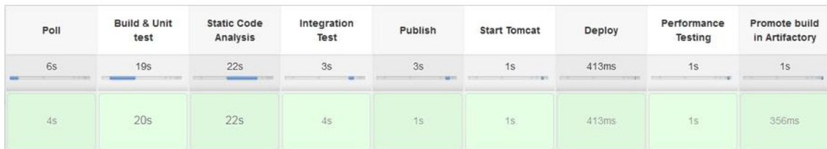
Jenkins CD pipeline in action
