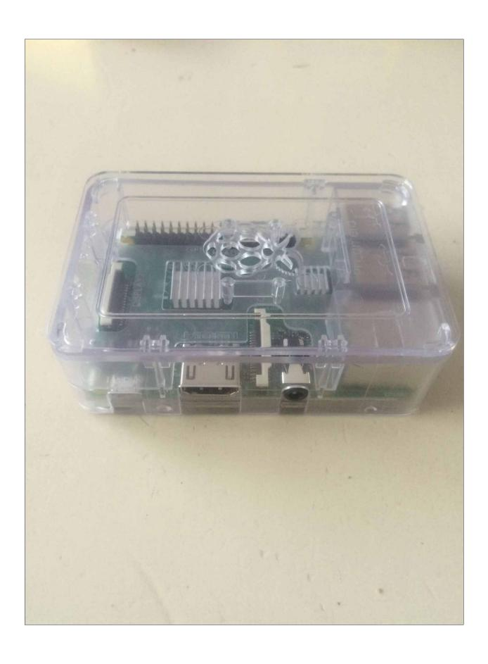
After that, the Raspberry Pi 3 was fully assembled, we merely hooked up our monitor via the **High-Definition Multimedia Interface** ( **HDMI** ) interface using the cable provided, which is plugged in our USB mouse and keyboard, and start preparing for the SD card for the operating system.
