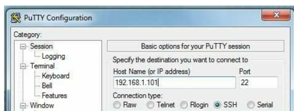
Figure 2: Configuring Putty to connect to the Pi
