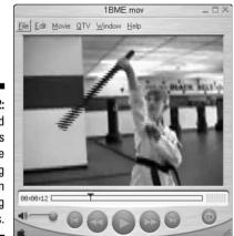
Figure 3-2: Interlaced cameras can cause interlacing jaggies on fast-moving subjects.
