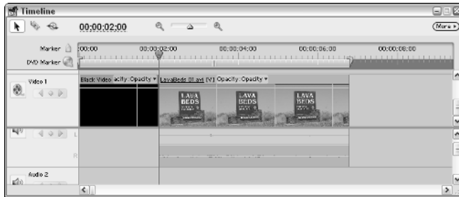
Figure 8-6: Insert edits insert clips between existing clips, shifting subsequent material to make room.
