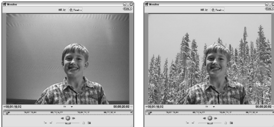
Figure 11-2: Use the Chroma key to remove an entire color from a video image.
