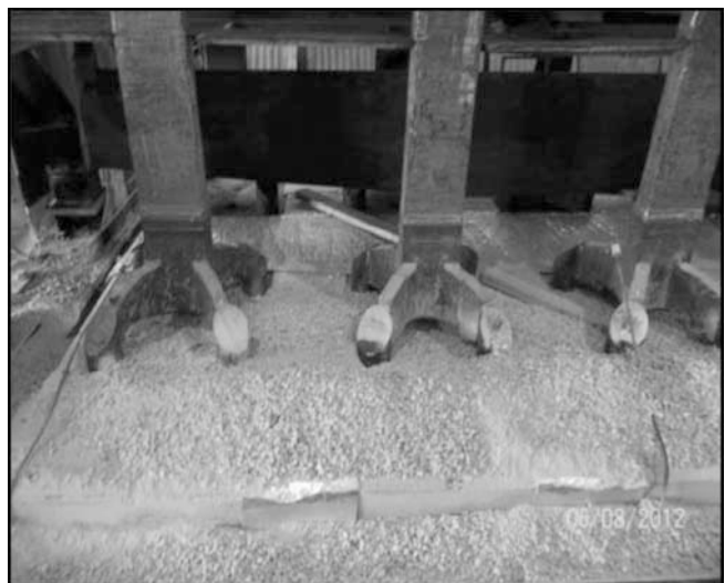
Figure 5. Crushed tapped bath in sidewall and on top of anodes.
