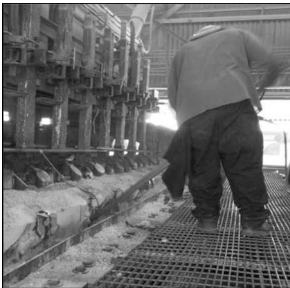
Figure 7. Dry bath pushed between anodes to melt. Note air-cooling pipes on anode assembly.
