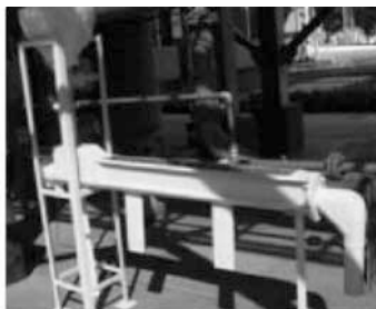
Figure 11 – Air-fluidized conveyor of 1.5 m long with three outlets - source [10].
