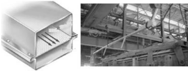
Figure 10 – The Albras aluminum smelter air fluidized conveyor and a conventional air slide in the left - source: [10].
