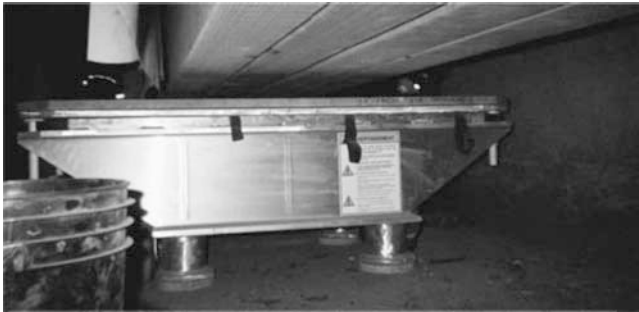
Figure – Floating Potential Lifting Table
