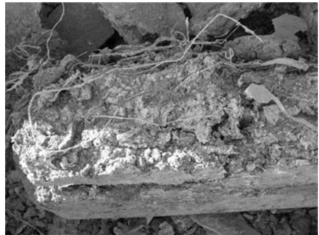
Figure 1. Steel wire embedded in white dross.
