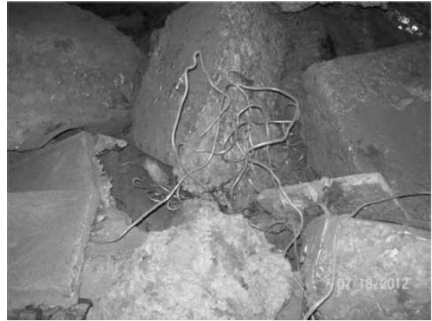
Figure 4. Grain refiner rod mixed in with dross.
