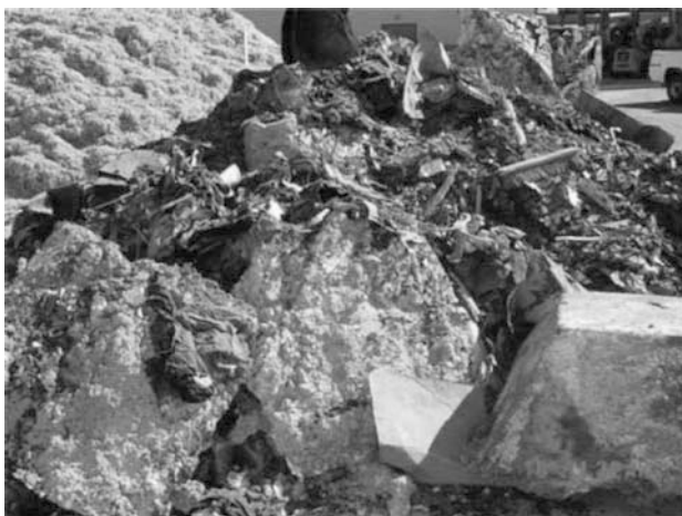
Figure 3. Garbage mixed in with dross.
