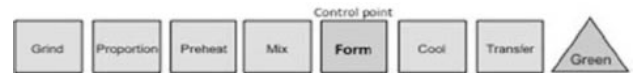
Figure 3. Process flow sheet for the Paste Plant showing Vibroforming as the control point.
