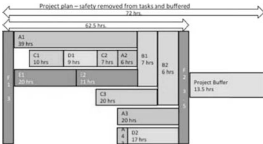
Figure 15. Repair timeline with revised task times and project buffer.
