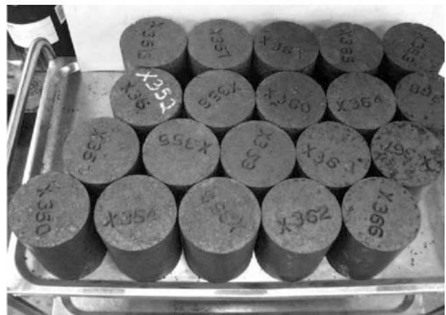
Figure 5: Five batches - each with four pilot anodes, individually marked. Mass is 3.80±0.01 kg/dm 3 . Over 1400 have been made in the last six years.
