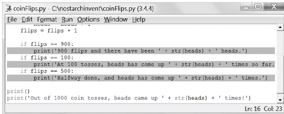
Figure 6-6: Three breakpoints set in coinflips.py
