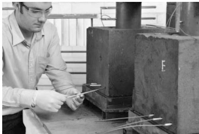
Figure 4. Wiring of the samples for voltage and temperature measurements.
