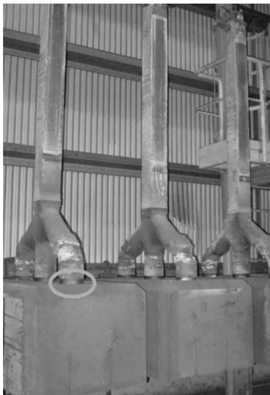
Figure 1. Typical anode rod assemblies ready for use in aluminium smelting (image used with permission of Century Aluminium). Stub to carbon (STC) connection highlighted.
