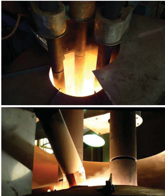
Figure 3. Photographs of the continuous feeding of the EAF with the dusty material mix, through a top lance feeder in the AoG pilot plant.
