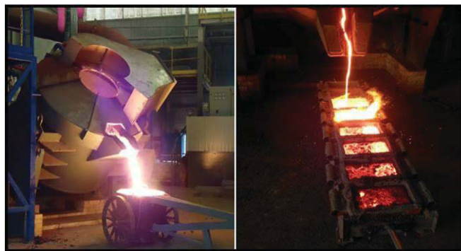
Figure 4. Pouring of slag (left) and metal phase (right) in the AoG pilot plant
