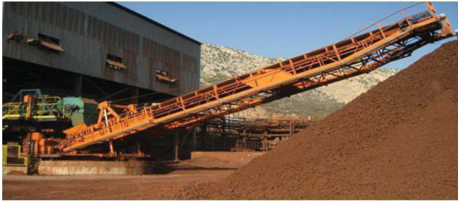
Figure 1. Dewatered BR exiting the filter presses in AoG
