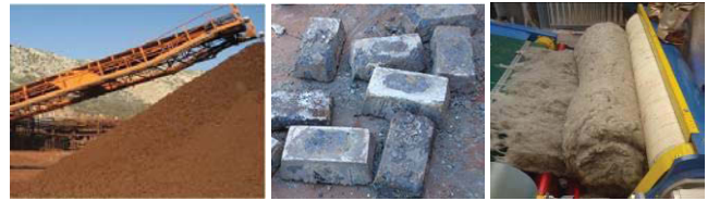
Figure 7. The ENEXAL BR treatment process in AoG; dewatered BR is transformed 100% to pig-iron ingots and mineral wool
