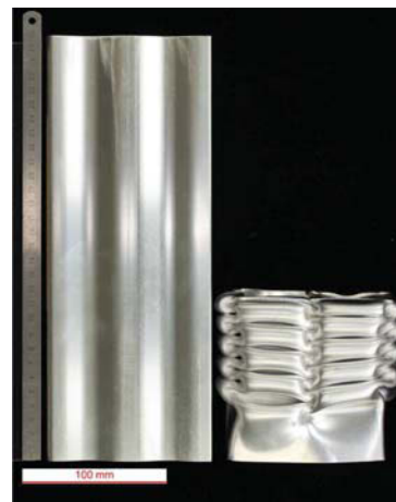
Figure 2. Profile before and after the crush test.
