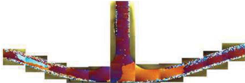
Figure 4. Profile microstructure after a heat treatment with 580°C/22h (variation 4).
