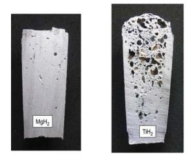
Figure 10. Examples of aluminium foam structures using MgH<sub>2</sub> and TiH<sub>2</sub>.
