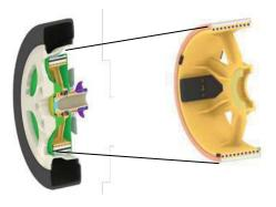
Figure 1. Wheel hub motor design (left: complete Wheel with motor; right: stator of the wheel hub motor), [3].
