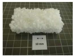
Figure 8. Example for a stable core consisting of bonded grains of salt.
