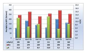
Figure 4. Mechanical properties of the AlSi8.5-alloy (conventional [Var. 1] and optimised alloy [Var. 5]; F=as cast; T5=180°C/2,5h; V=180°C/120h)
