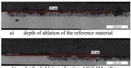
b) depth of ablation of optim. AlSi8.5Mg-alloy
