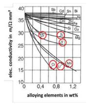
Figure 2. Influence of the alloying elements on the Electrical conductivity, [4].
