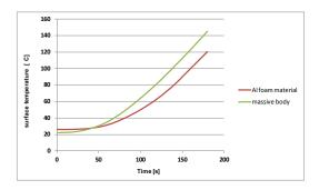
Figure 11. Comparative temperature measurement between a sample made of aluminium foam sandwich and a massive body sample
