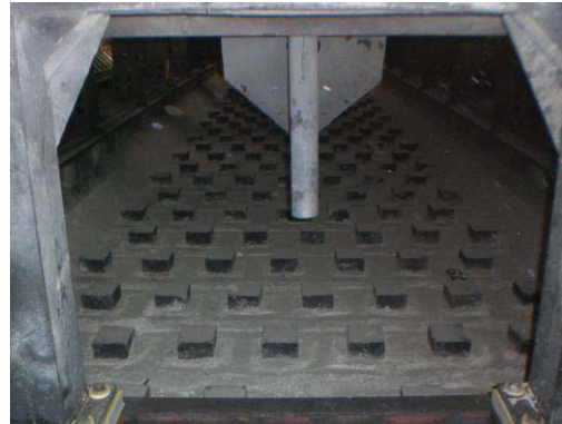
Figure 1. Aluminum reduction cell with innovative cathode.
