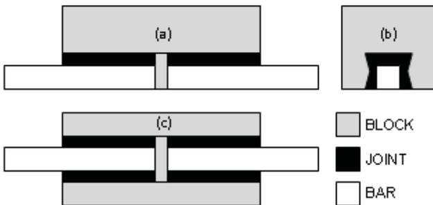
Figure 1. Sketch of typical cathode block assembly: (a) side cut away, (b) end view, (c) bottom view.
