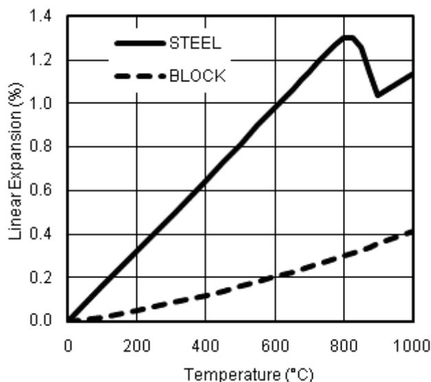
Figure 7. Nominal linear thermal expansion for a carbon steel collector bar and a carbon cathode block. Note the contraction of steel starting near 800 °C.
