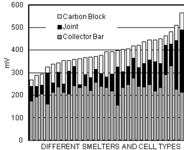
Figure 2. CVD components for different plants, cell technologies, and joint materials. Joint contact voltage was determined by tuning a model's joint contact resistivity to make the calculated CVD match each plant's measured CVD. The averages of all joint voltages and resistivities are 100 mV and  $10 \Omega\text{mm}^2$ , respectively. No clear advantage between different joint materials was evident.
