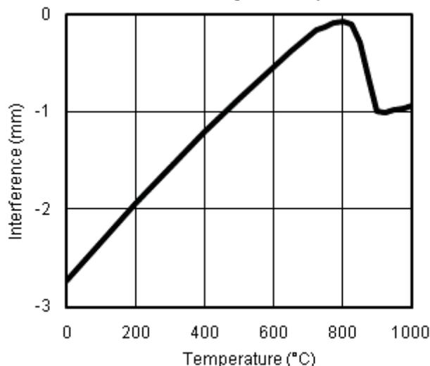
Figure 8. A representative calculated interference fit between the width of a carbon steel collector bar and a carbon cathode block. Note the loosening as interference drops above 800 °C. In this example all values are negative, i.e. no interference.
