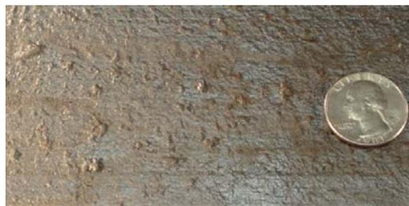
Figure 9. Example of cast iron texture on the surface that solidifies against the carbon slot in a cathode block.
