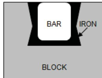
Figure 3. The cathode assembly, upside down for rodding. In most practices, cast iron does not cover the bar, resulting in undesirable asymmetric heating of the bar by the hot iron.
