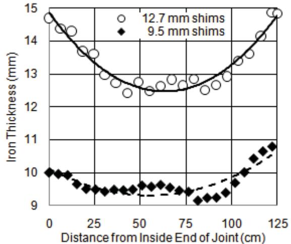
Figure 6. Autopsies of unused cathode assemblies showed anticipated longitudinal thinning of the iron.
