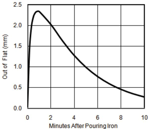
Figure 5. Predicted out of flatness due to bowing of a collector bar after pouring cast iron.
