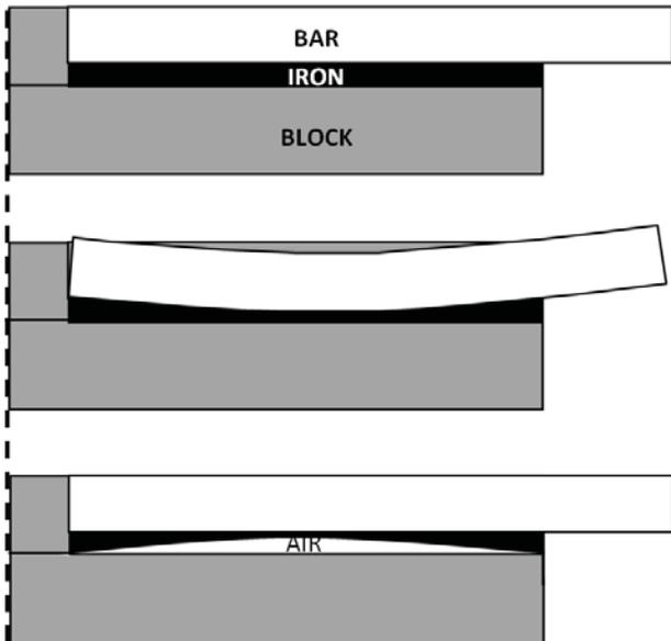
Figure 4. Half of bar-block assembly. Molten cast iron heats the bottom of the collector bar (top). The iron freezes with the bar bowed up at its ends (middle). As temperature evens out the bar straightens leaving a lens shaped air gap (bottom).
