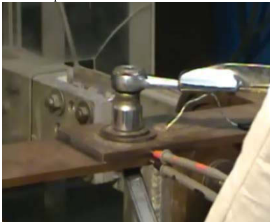
Figure 8: 10X10 cm, Cu/Cu contact
