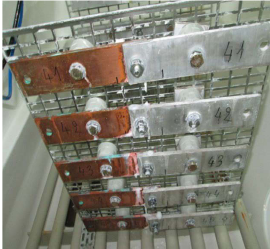
Figure 2: Salt mist and humidity to test the metallic foam
