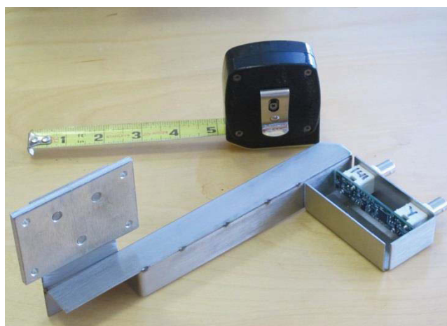
Figure 1: A "slave" (to the right of the photo) mounted within its enclosure. The flange on the left is attached to the bus and the reinforced "arm", to the right of the flange, places the slave behind an anode rod. Photograph before the slave is insulated.
