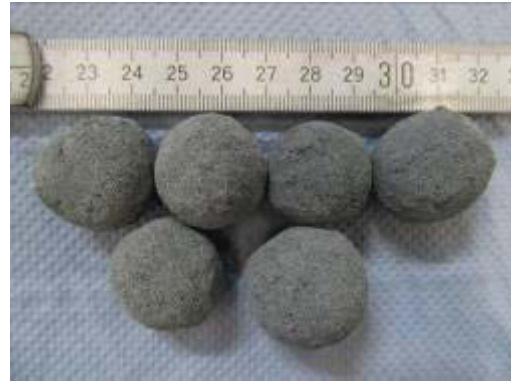
Figure 5: Alumina wood-charcoal pellets used in experiments.
