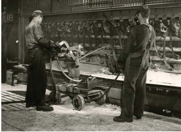
Figure 1. Breaking a hole in the side crust of a HS Söderberg cell at the Alcan Arvida smelter in 1944. Source: Rio Tinto Alcan
