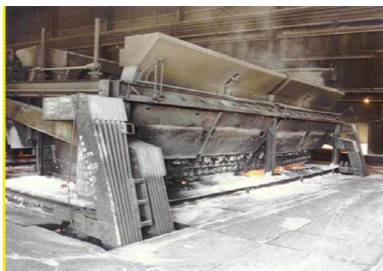
Figure 3. A 150 kA side-by-side HS Søderberg cell at the Reynolds Arkadelphia smelter in the 1980s.
