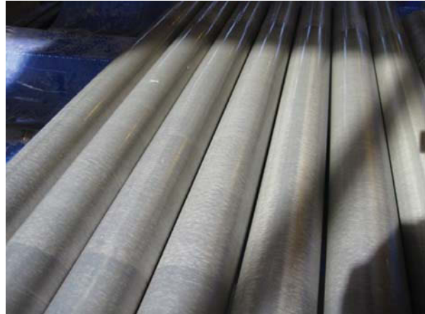
Figure 10. AA2024 billets cast with the LPC casting technology.
