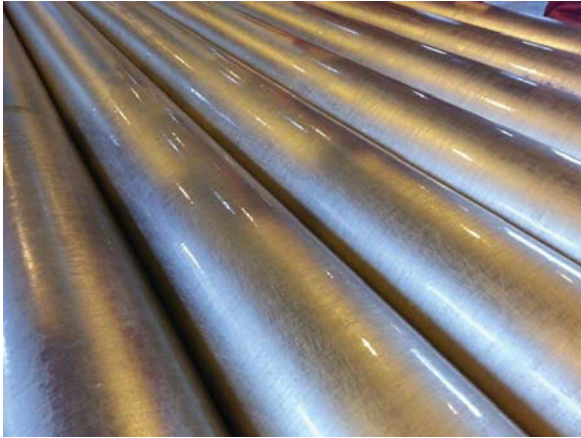
Figure 13. AA707 billets cast with the LPC casting technology.
