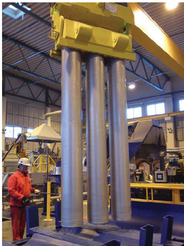
Figure 1. Ø405mm (16") LPC billets just after casting, AA6060 alloy.
