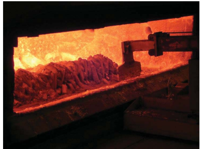
Fig. 13: Push of primary ingots 1h after charging in a remelting furnace.
