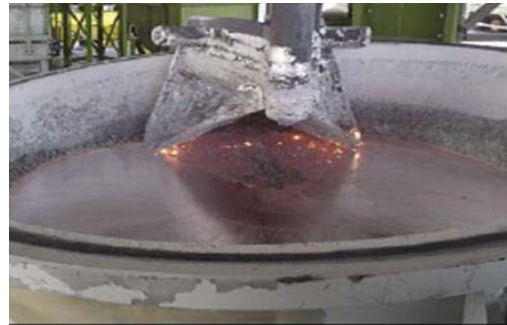
Skimmer at TAC station
