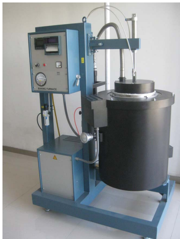
Figure 3. Anode Baking Furnace.
