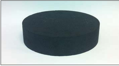
Fig. 10: Photography of the green compact, pressed in laboratory.
